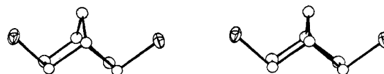
Figure 3.—ORTEP stereodiagram of \beta\text{-P}_4\text{S}_3\text{I}_2 showing the orientation of the ellipsoids of thermal motion of the iodine atoms.
